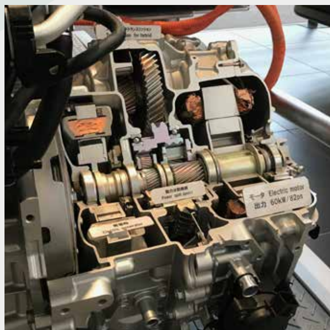
Figure 98: Toyota Prius generator and motor.
