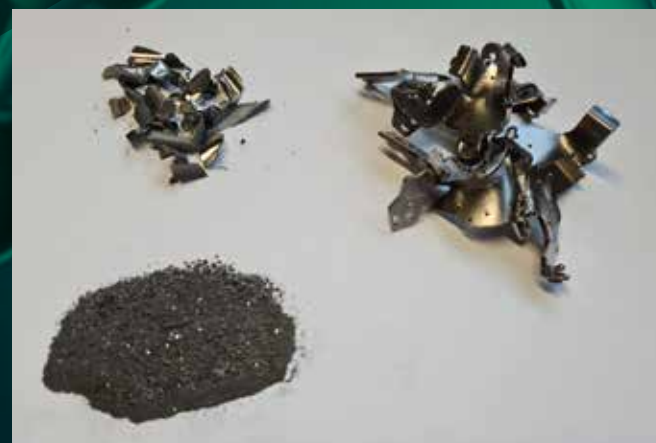
Figure 109: Voice coil magnets after HPMS processing
