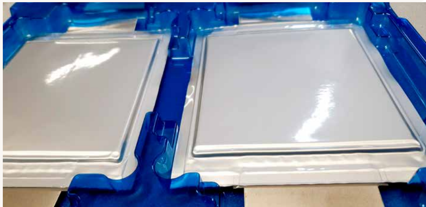
Figure 30: One type of Lithium-ion battery, the pouch cell, used in automotive applications. In the section on secondary materials, Figure 112, there is some additional explanation of different automotive battery form factors.
