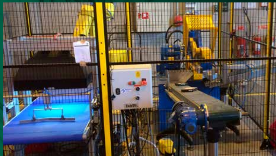
Figure 107: Automated handling and separation of voice coil motor from hard disk drives. Developed as part of the REMANENCE project.
