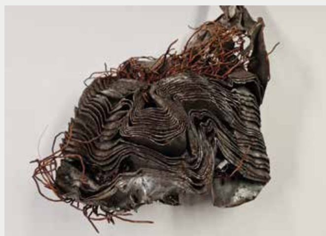
Figure 100: Rotor from an electric motor after shredding
