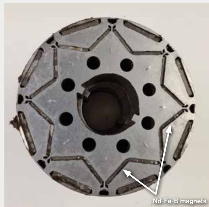
Figure 99: Rotor from an electric motor with glued Nd-Fe-B magnets.
