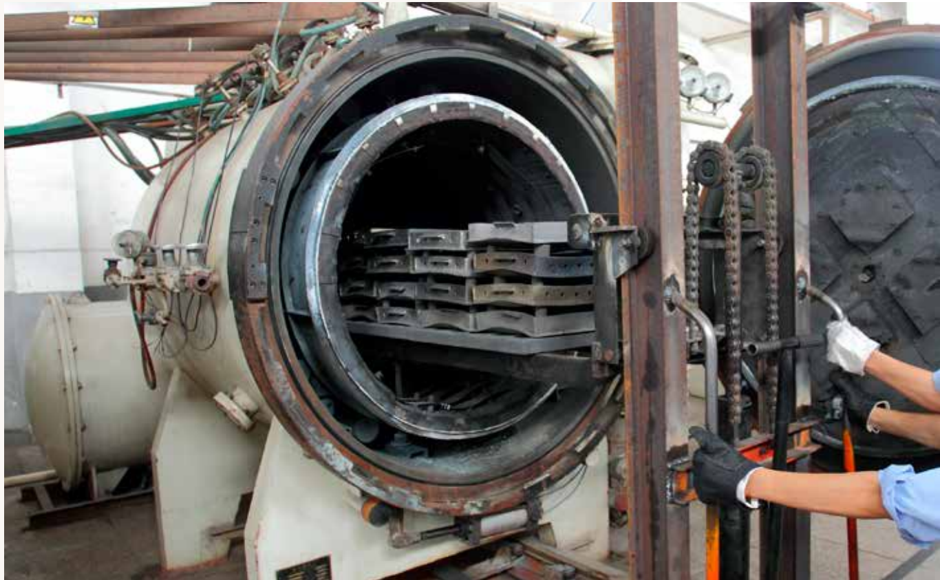
Figure 25: Sintering of Nd-Fe-B magnets
