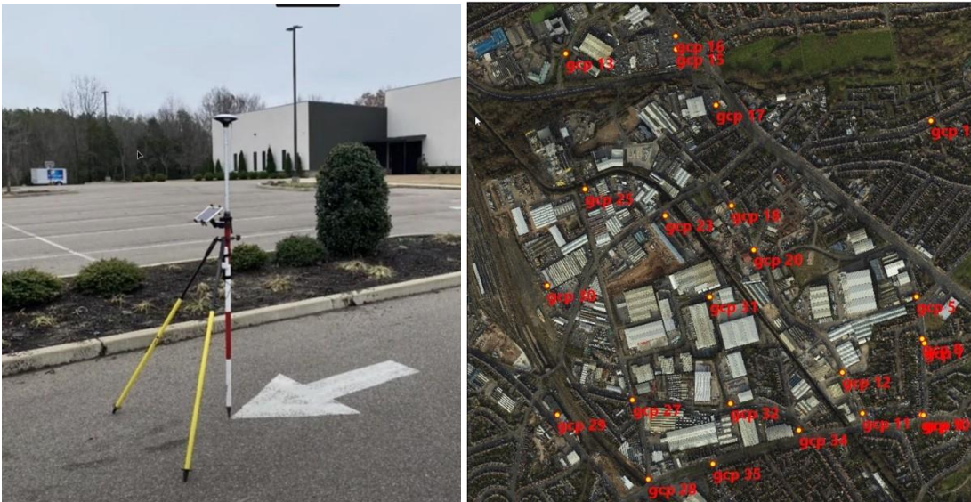
Figure 4: Distribution of the control points on the Image layer of the ortho projection
