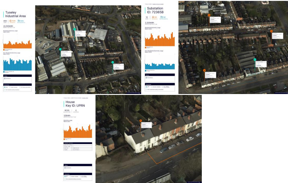
Figure 5: Screen shots from demonstrator, consisting of 3 levels: Area, Substation, Building and 4 scenarios: Base, Electric Vehicle adoption, Increase in Energy Performance Certificate rating, Industry PV adoption.
