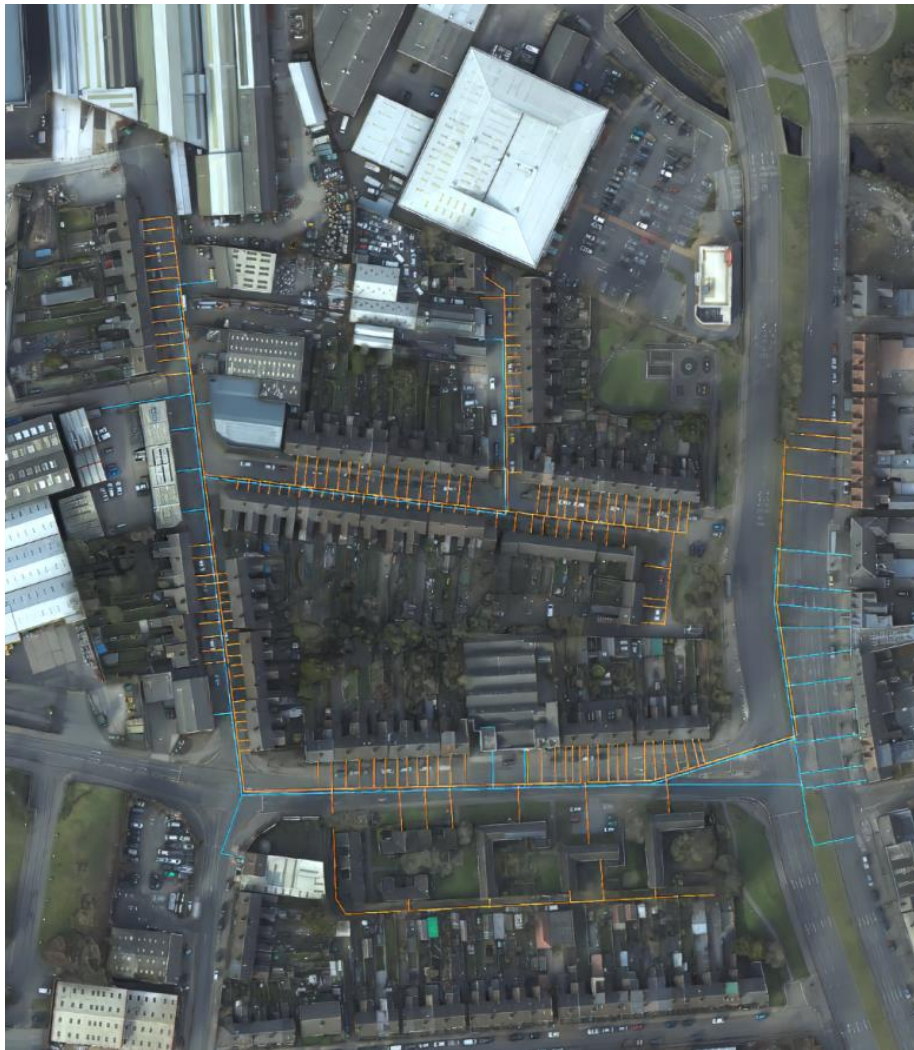
Figure 8: Aerial scan of part of TEED with residential (orange) and non-residential (blue) substation electrical flows visualised.
