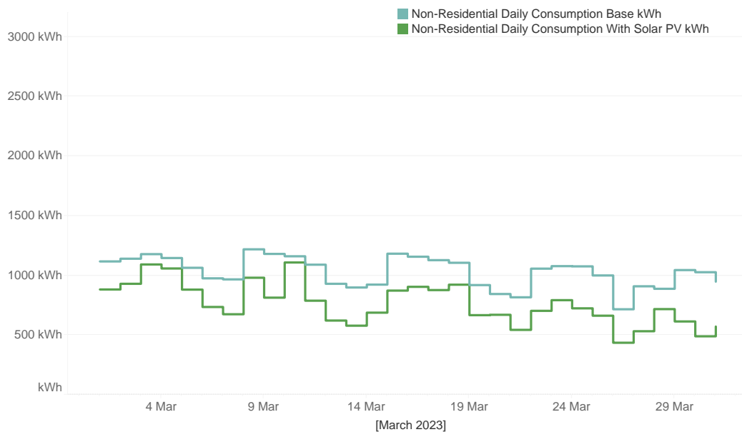
Figure 16: The total daily electricity demand for the non-residential properties in Kings Road, LV substation area in the baseline scenario (above) and in the solar PV scenario (below).
