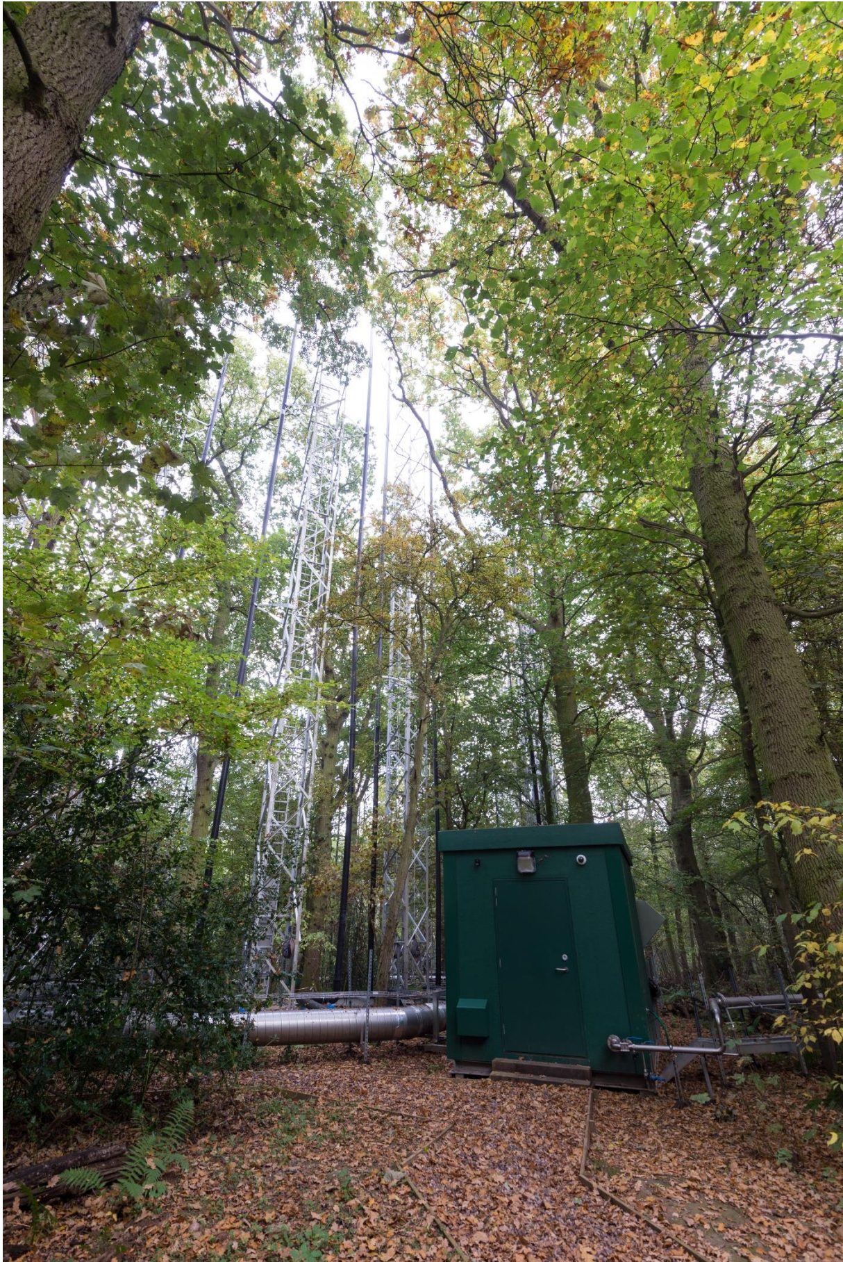
Figure 11 each mast is 25m high and each array is 30 m in diameter
