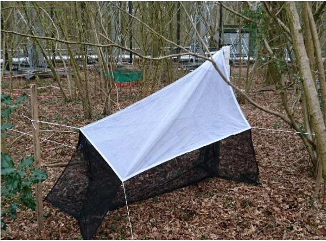
Malaise trapping forms part of the monthly invertebrate sampling which contribute to the long-term ecological measurements taking place at the site
