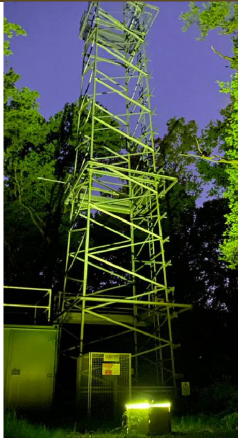
The flux tower at BIFoR FACE, lit up at night by a moth trap. Photo credit: Gael Denny, Technician.
