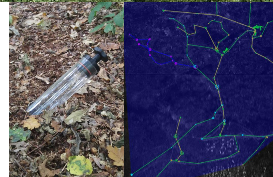
Figure 3: Left: a minirhizotron installed in an array. Right: a root image analysed using SmartRoot [3]
