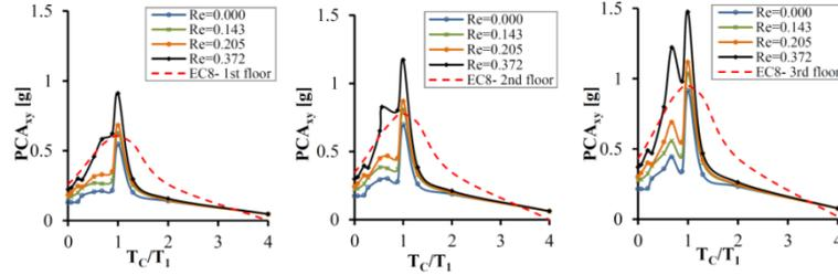
Fig. 4 Comparison between the FE results and EC8 for NSCs attached to P-structures at: (a) first, (b) second and (c) top floors.
