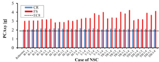
Fig. 6 Comparison between the FE results and EC8 for NSCs attached to P-structures having different cases of vertical mass irregularities.
