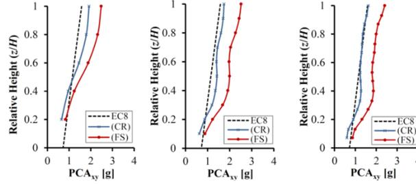
Fig. 2 Comparison between the FE results and EC8 for NSCs attached to P-structures having heights equal to: (a) 15, (b) 30 and (c) 45 m.
