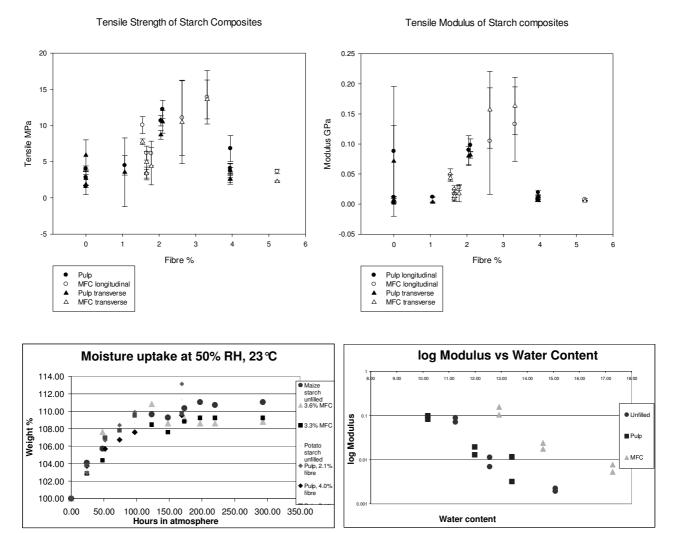
Clockwise: Tensile Strength vs filler content, Young's modulus vs filler content, modulus vs mass released on heating to 170°C, mass increase on conditioning at 50% RH
