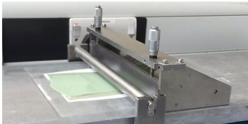
Figure 5: Reverse tape casting consist of electrolyte, anode functional layer and anode substrate layer
