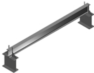
Figure 3. Simply supported beam.
