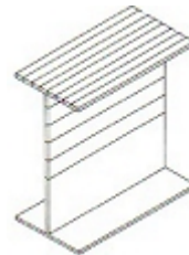
Figure 4. I-Beam divided by strip method.
