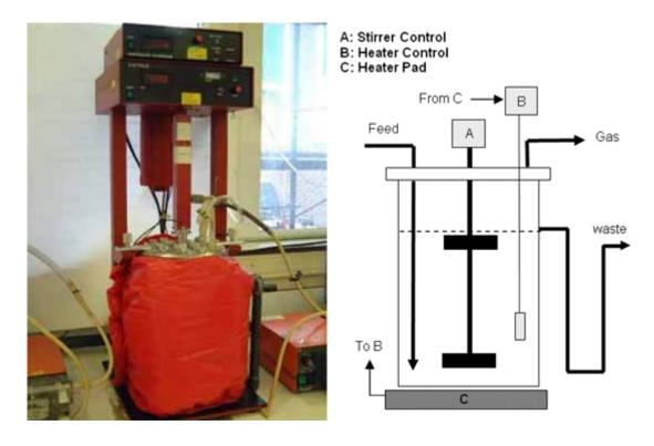
Figure 1 Photograph and schematic diagram of the bench-scale digester
