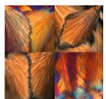
A 'trouble maker' from a bygone method of glass production could find a new use as an optical diffuser in medical laser treatments, communications systems and household lighting. A form of crystal that was long considered an unwanted and unloved 'stone' in glass making could find practical use as a cheap and efficient optical diffuser, which are used to scatter and soften light for a range of industrial and household applications. Read more.
