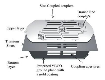
The Butler Matrix is constructed of two  $LaAlO_3$  single crystal substrates with superconductor on both sides. All four layers of superconductor are patterned and are bonded together with a 50 micron thick titanium sheet which acts as the ground connection. The construction allows microstrip circuitry on the upper and low sides of each substrate, with coupling of the microwave signal through the ground plane. This gives a much reduced size to the device.
