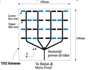
substrate. The patterning is on both sides of the substrate. Short dipoles with parallel strip transmission line feed networks are used.
