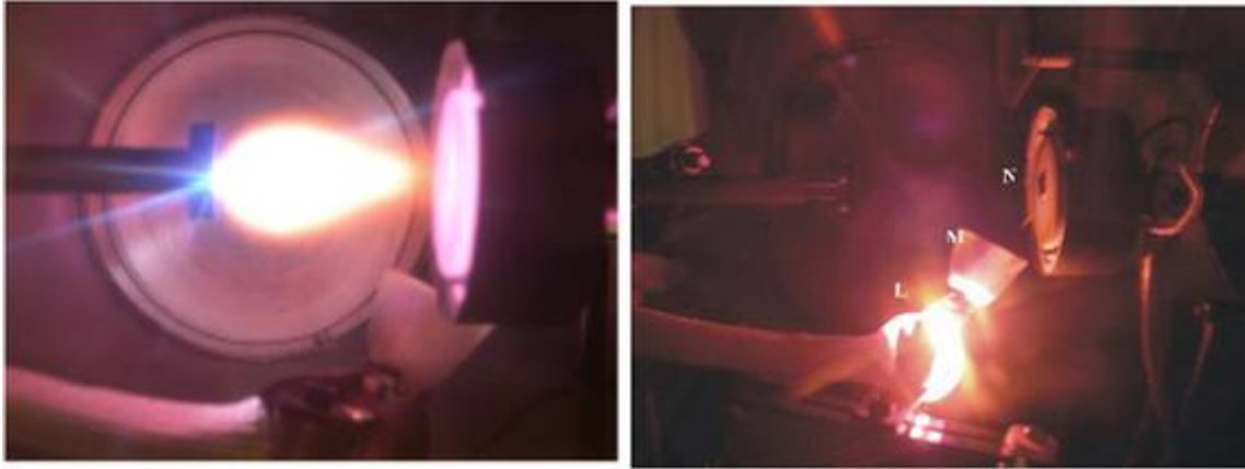
Figure 4 Left pulsed laser deposition of YBCO. Right in-situ thermal evaporation of gold
