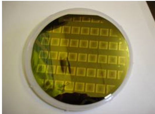
Figure 3. A 4 inch silicon wafer is used as a support for the polyimide substrate for and array of gold test structures.
