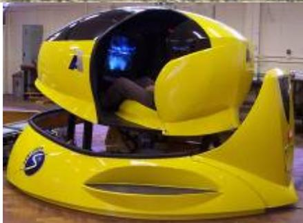
project resulted in the development of a vibration sensing device which was flown on an EC-203 helicopter whilst performing a range of typical marshalling manoeuvres. The data collected were then used to drive a 3-axis modified entertainment simulator motion base, linking the simulator motion and vibration to interactive 3D graphics developed using Microsoft's *Flight Simulator 2004*. A more permanent control system supporting the integration
