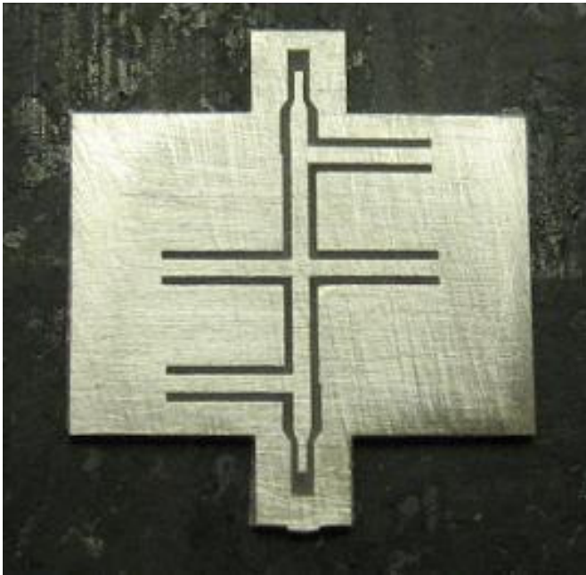
Figure 1 Electroformed Nickel Millimetre Wave Microcomponent [1].
