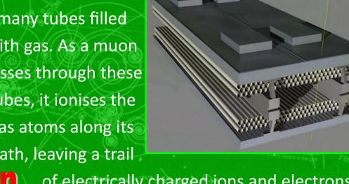
of electrically charged ions and electrons which drift to the central wire where they're measured. By measuring the time it takes for these particles to drift to the wire, its possible to determine the path of the original muon as it passed through the chamber.
