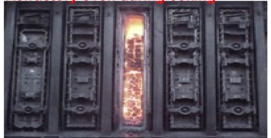
Refractory oven during coking
