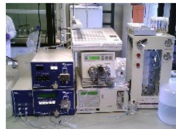
Particles of varying sizes (more correctly diffusion coefficients) are separated by their interaction with a parabolic velocity gradient within the channel and a secondary force (a secondary flow in this case) applied perpendicular to the channel flow. Particles are pushed towards a so-called accumulation wall and the concentration gradient set up encourages back diffusion into the channel. The smallest (most diffusive) particles diffuse into the highest velocity flow and are eluted first.
