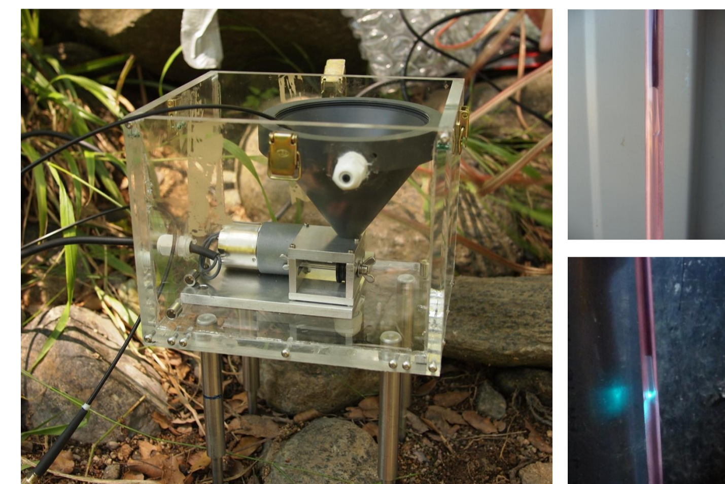
Fig. 2: Prototype of the miniDOS prior to installation in situ . Left panel: control unit (not shown here: battery, fiber optic oxygen transmitter, battery). Right panels: side-firing POF in tubular oxygen probe.
