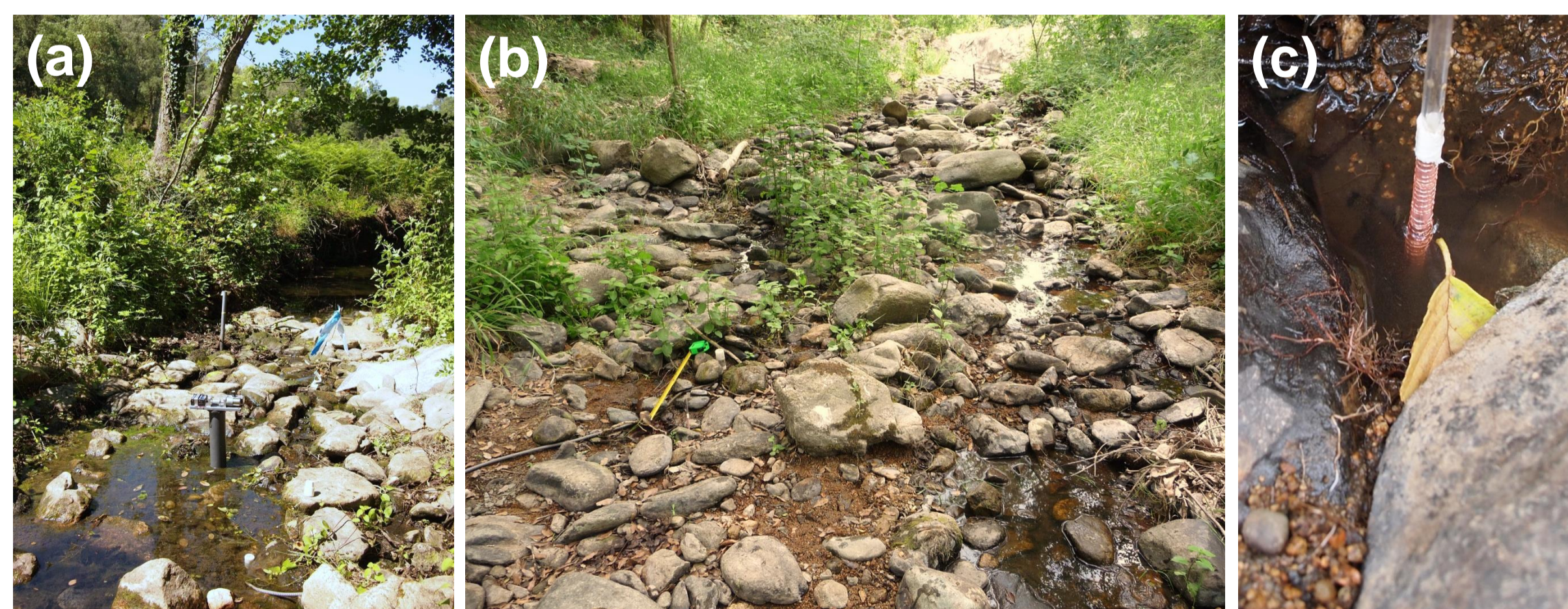
Fig. 1: Locations of repeated DO measurements in the HZ of the Fuirosos stream: (a) upstream and (b) downstream of pool-cascade sequence with (c) tubular oxygen probe installed in the streambed
