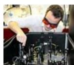
GEES researchers have used a laser beam trap to examine how drug particles from asthma inhalers behave as they are projected through the air. Their findings could improve the effectiveness of inhalers for the 5 million people in the UK suffering from asthma.
