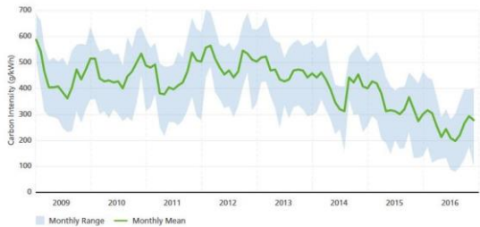
Figure 5.4 The carbon intensity of British electricity, showing the average and range for each week [187].
