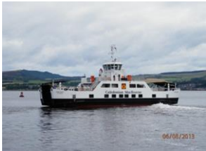
CMAL's MV Hallaig diesel-electric hybrid ferry undergoing sea trials in August 2013
