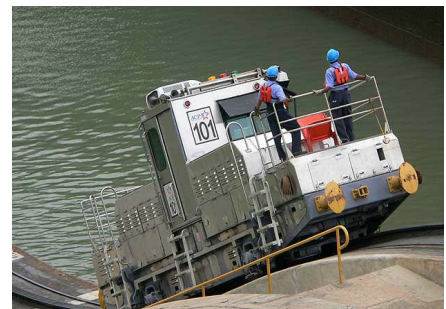
Figure 2 Panama Canal Tug Locomotive on Rack Section (Picture Wiki Commons)
