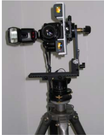
Figure 1: Prototype image collection system, showing camera, flash and distance measurement lasers.
