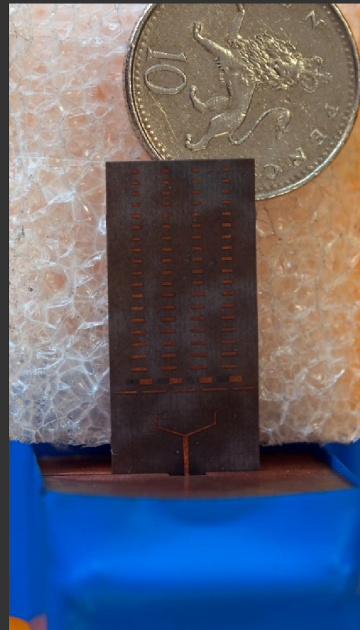
Printed Yagi-Uda array gain ~20 dBi
