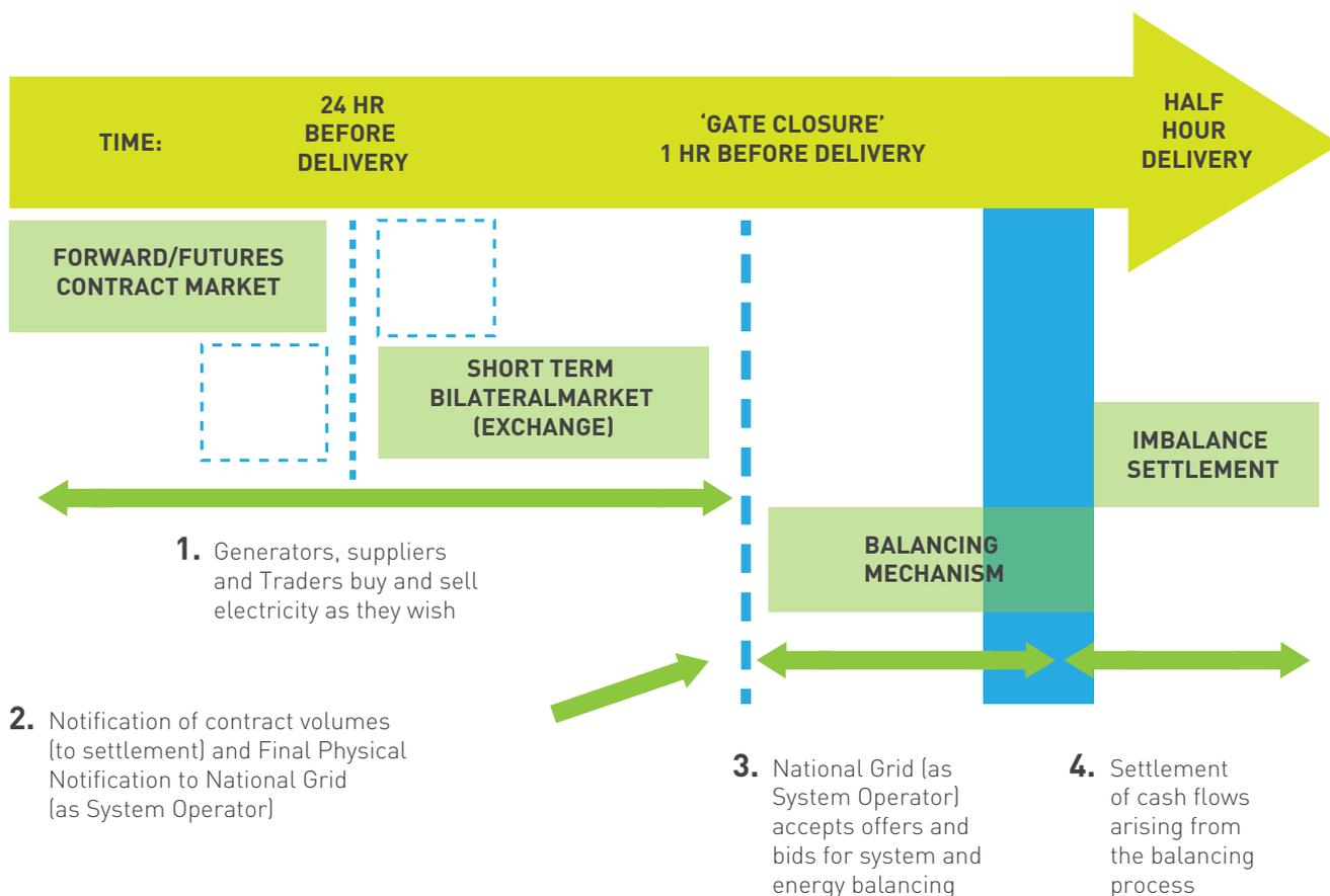
Figure 4.1 The British Electricity Trading Arrangements.
