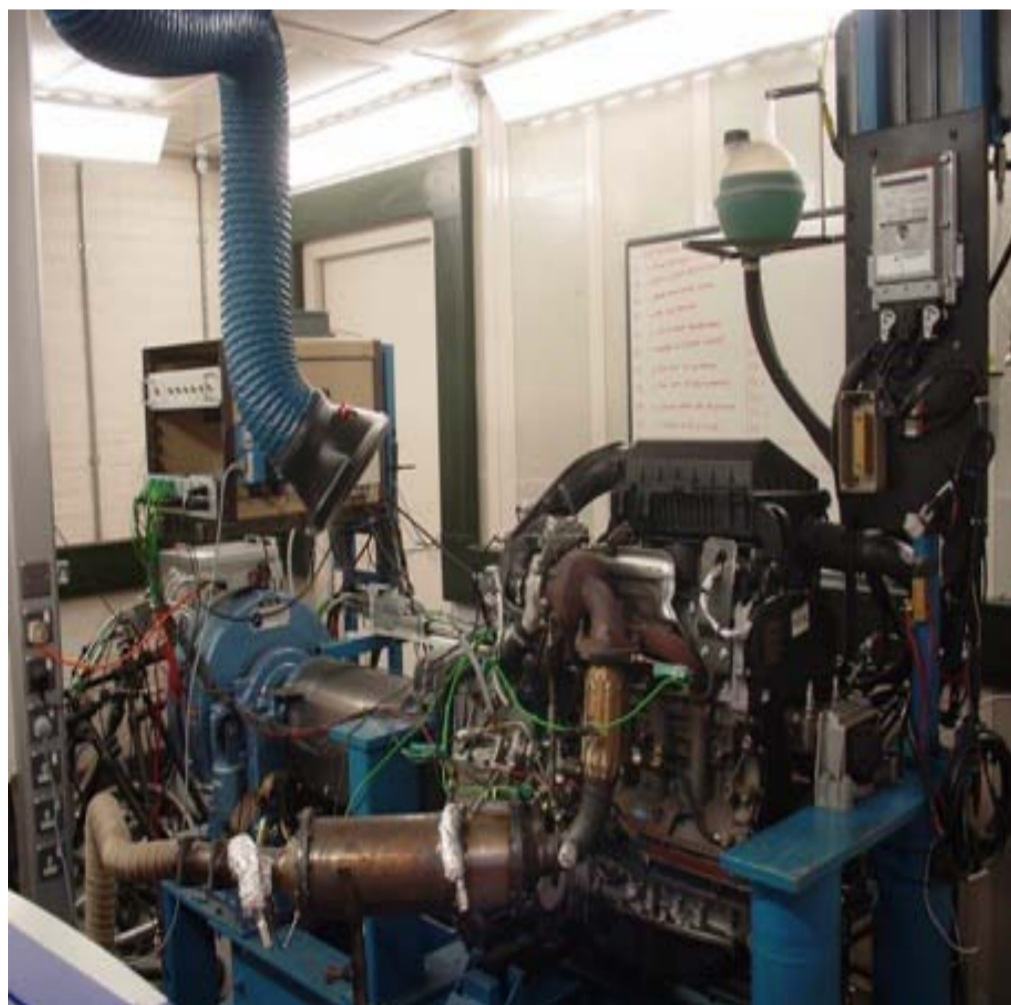
Figure 1 Ford Puma engine test rig
