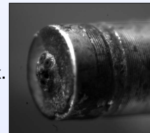
Figure 5 GDI Injector Tip Deposits
