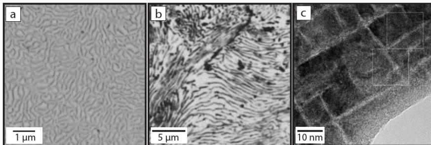
Micrographs of high temperature 'bcc superalloys' based on Ti-Mo [2] Cr-W [4] and TaNbHfZr HEA [5] that this project seeks to extend to tungsten alloys.
