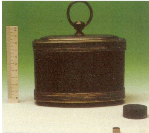
Figure 1b: Brass bound lodestone, ferrite block and NdFeB magnet: each store the same magnetic energy (~0.4J) & contain ~70% iron by weight, yet the mass has decreased a thousand fold.
