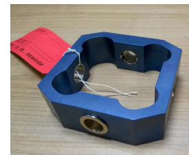
Component 3. Gimbal for UTAS from Ti6Al4V
