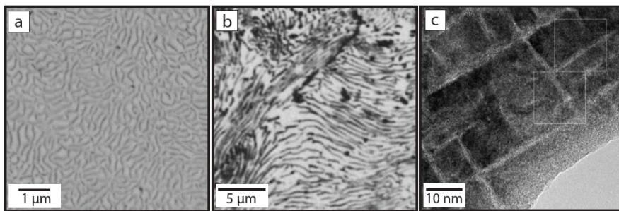
Micrographs of high temperature 'bcc superalloys' based on Ti-Mo [2] Cr-W [4] and TaNbHfZr HEA [5] that this project seeks to extend to tungsten alloys.
