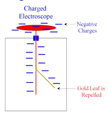
Electroscope would discharge much faster at higher altitude
