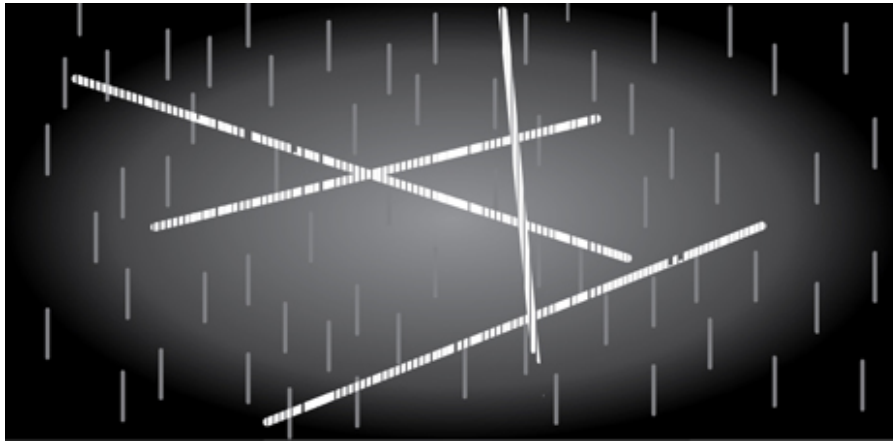
Figure 3: These tracks confirm the presence of muons . Like electrons, muons are leptons however they have a greater mass. As they are heavier than electrons, they are not so easily displaced by air molecules resulting in a long straight track. You may be lucky enough to see these tracks as they are not very common. These muons are produced by cosmic rays interacting with our atmosphere. If you would like to know more about cosmic rays, go to the appendix of this document.
