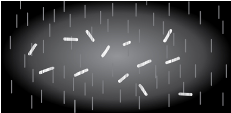
Figure 1: Short fat tracks show the presence of alpha particles . In comparison to other radiation, alpha particles are heavy as they are made from 2 neutrons and 2 protons (the nucleus of a helium nucleus). Due to their size and low energies they do not travel far and therefore produce short tracks.
