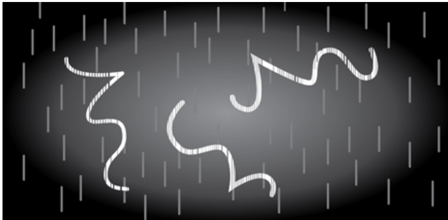
Figure 2: These unusually shaped tracks are produced by beta particles , better known as electrons and/or positrons. A positron is the anti-particle to an electron and has the same mass but the opposite charge to its sister particle. As electrons are much lighter than alpha particles, we see longer tracks. The unusual pattern is as a result of being bounced around by heavier air molecules.
