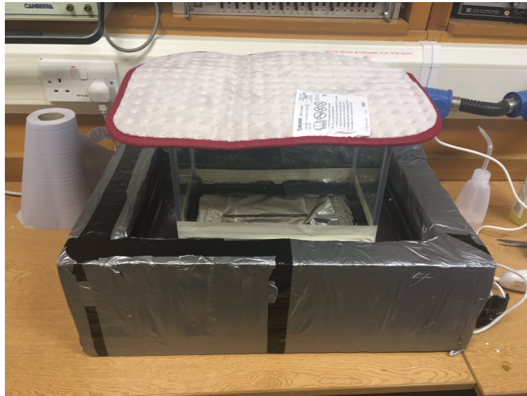
Figure 16: Cloud chamber set up with electric blanket. Can also be created with a hot water bottle or without any heating.
