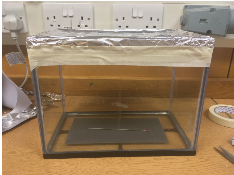
Figure 12: The tinfoil taped to the fish tank making the tank air tight.
