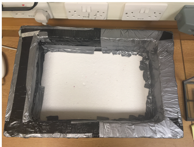
Figure 6: An example base from a top view. Top of base (rectangular ring) has dimensions 10cm deep and 5cm wide around long edges and 7cm wide around short edges.
