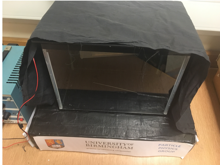
Figure 8: Final set up of cloud chamber with black cloth to increase visibility of particle tracks.
