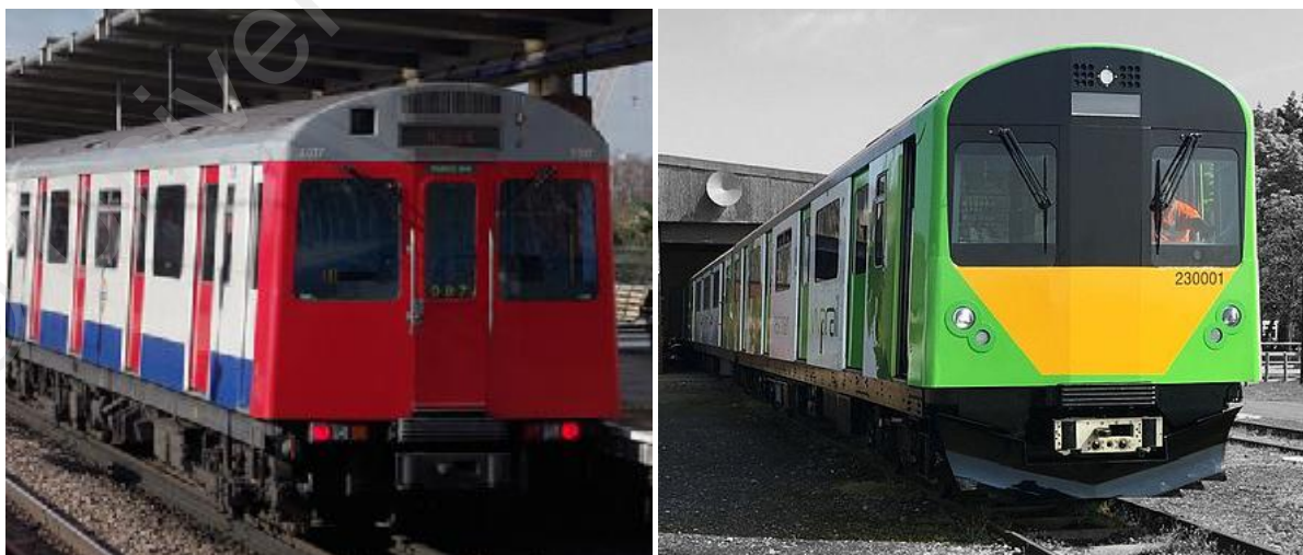
Figure 12 – D-stock to Class 230 conversion: before (mattbuck) and after (Alice Gillman)
