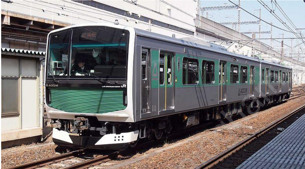
Figure 13 – JR-East battery-powered EMU EV-E300 set V1 at Utsunomiya station (Comyu)
