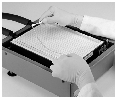
Fig 54. Positioning equilibrated Immobiline DryStrip gels on Multiphor II unit such that the anodic (acidic) side of the strip is toward the front edge of the gel.
