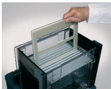
Fig 44. Loading the gel cassettes into Ettan DALT twelve electrophoresis unit.
