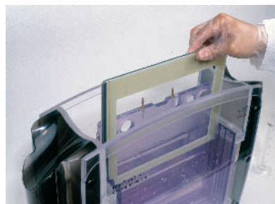
Fig 42. Inserting the cassettes into the cassette carrier.
