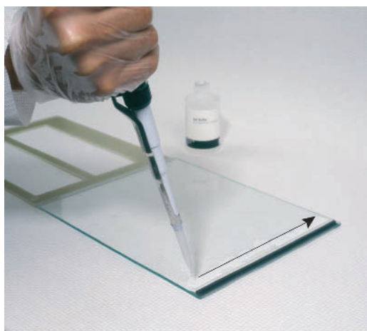
Fig 36. Pipetting a streak of gel buffer onto the glass plate. The arrow indicates the direction of motion in applying the streak.
