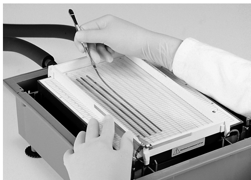
Fig 48. Positioning Immobiline DryStrip gels in the Immobiline DryStrip aligner.
