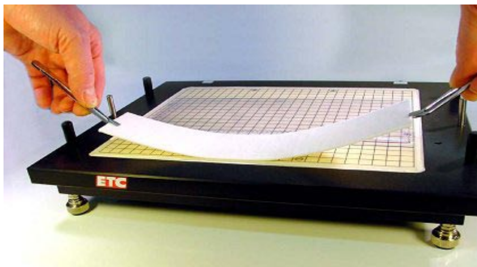
Figure - Applying a pre-soaked electrode wick to overlap the edge of the gel.
