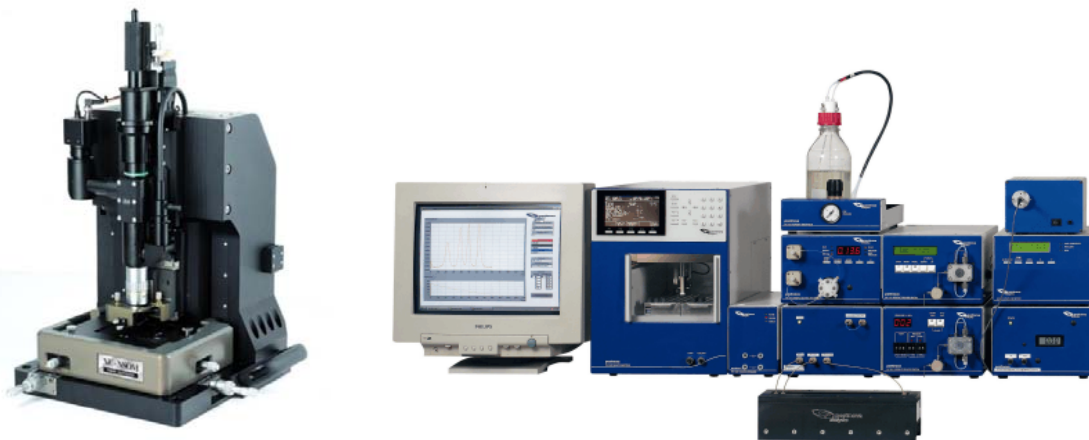
Figure 1. Images of atomic force microscope and flow field-flow fractionators used by FENAC, as part of a multi-method approach to nanomaterial characterisation. The AFM is housed within an environmental chamber reducing noise and allowing variable atmospheric conditions. Work is performed in air or liquid. The FIFFF is non-destructive and size selected eluents can be analysed by microscopy, for elemental composition etc. Both instruments have sub-nm resolution and can be coupled to provide morphological particle data (shape and permeability).
