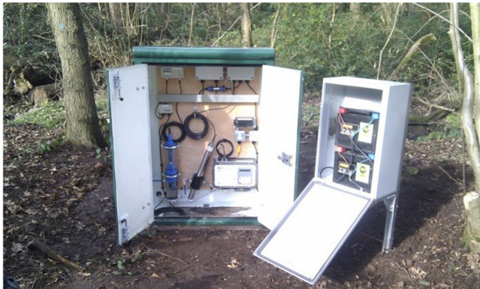
Fig. 3. Monitoring kiosk with Manta 2 (left) Opus (centre) and ISCO pump sampler head (right).
