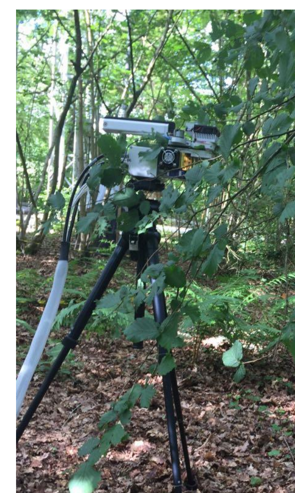
Picture 1: Measuring photosynthesis with a LI-6400XT gas exchange system (left panel), cutting-down oak branches from the upper canopy for photosynthesis measurements (right panel)
