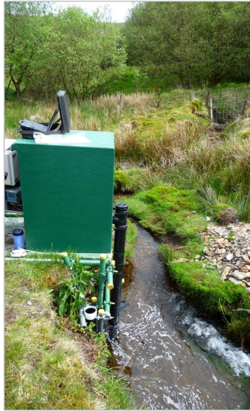
PVC pipe housing WQ sensors at LI8
