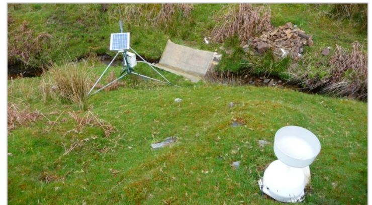
Tipping bucket rain gauge and flume at LI6
