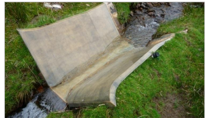
Fibre glass trapezoidal flume at LI6
