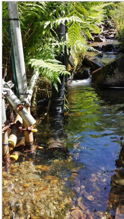
PVC pipe housing WQ sensors at LI6
