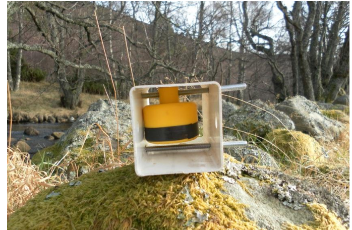
10 water temperature loggers
