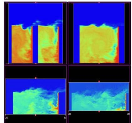
Fig. 1 Simulated flow & dispersion in street canyons with various street widths from the large-eddy simulation model at Birmingham.
