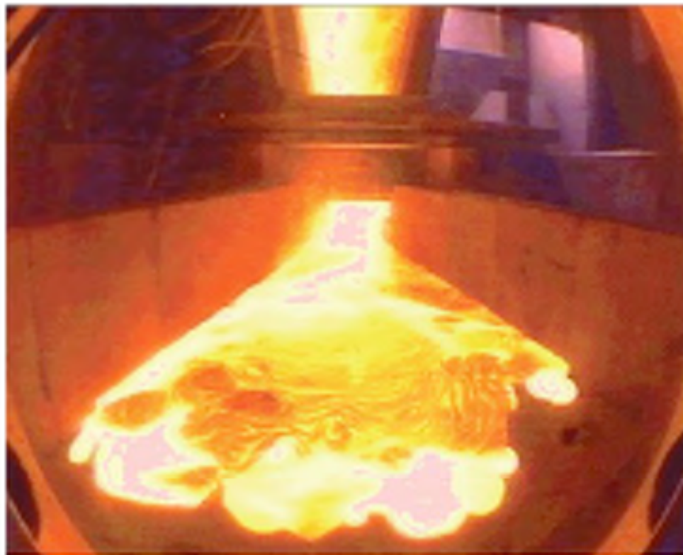
VULCANO (real \text{UO}_2 with some \text{Zr O}_2 )
