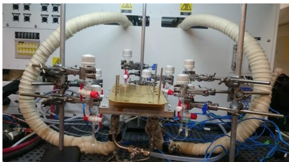
The test stand, showing insertion of the electrodes through the end plate.
