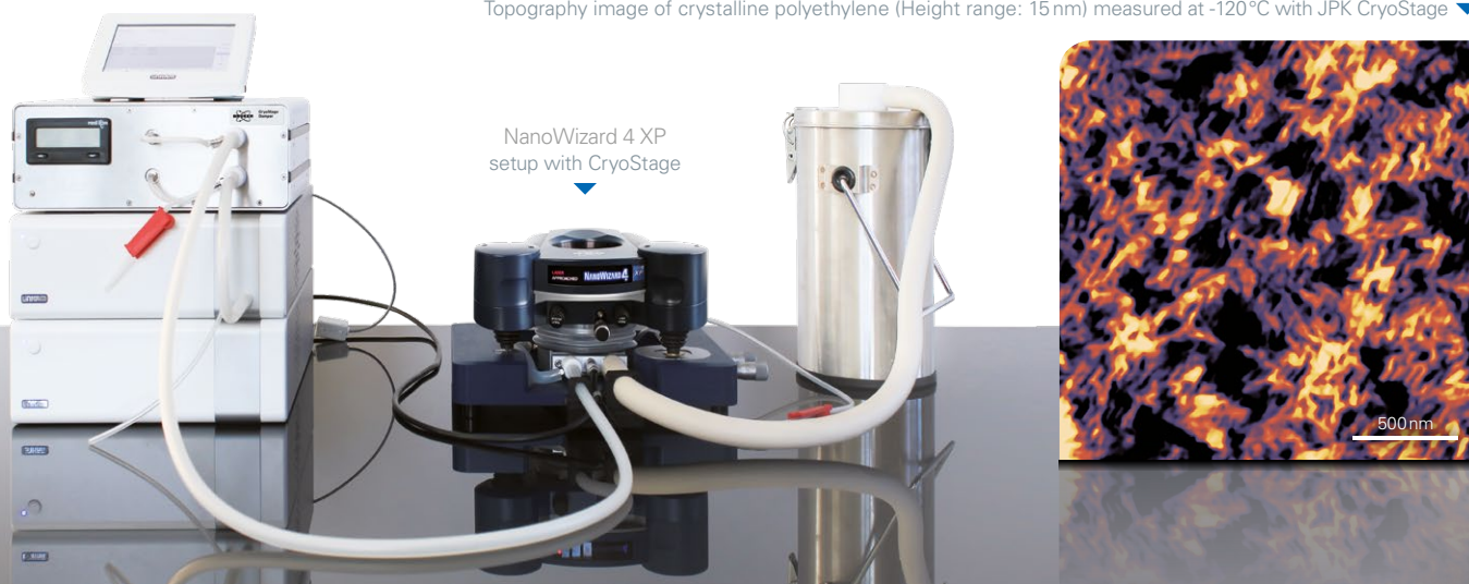
Topography image of crystalline polyethylene (Height range: 15 nm) measured at -120°C with JPK CryoStage
