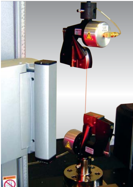
▲ Cord and yarn grips and AVE non-contacting video extensometer testing nitinol wire
