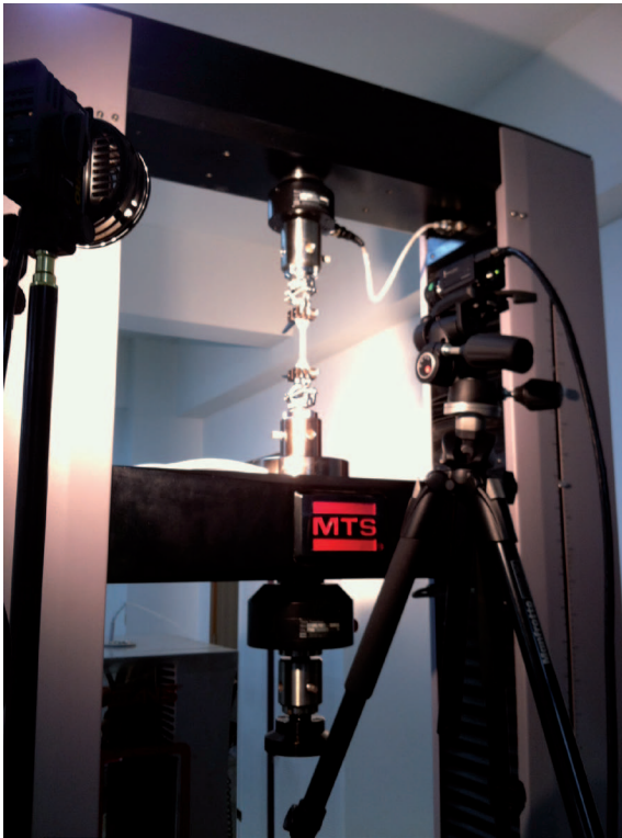
Laboratory tests on the edge seal of double glazing units
