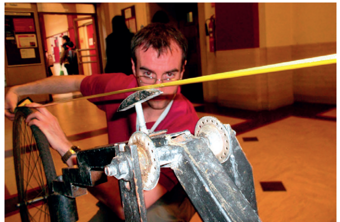
Roughness is measured on the university road network using TRL's MERLIN tool
